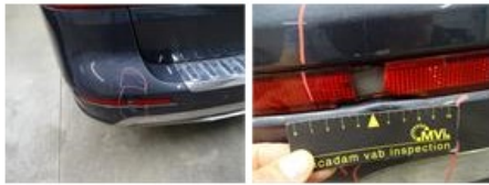
Bumper moulding F M, Broken, E - Replace
