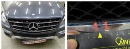
Bumper moulding R Mid, Dent(s), E - Replace
