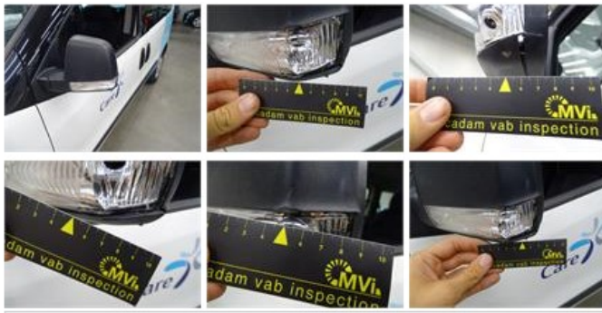
Wing F L, Scratch(es), LI - Repair and paint (complete)
