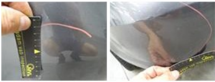
Bumper F, Deformed / Strained, LI - Repair and paint (complete)
