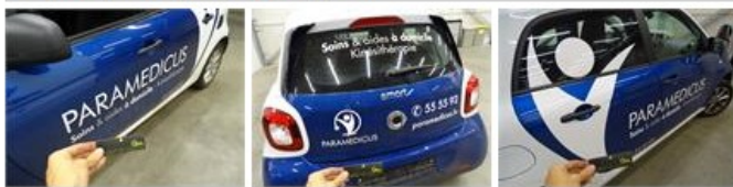
Door R R, Dent(s) and scratch(es), LI - Repair and paint (complete)
