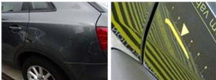
Trunk lid covering R, Scratch(es), Smart repair
