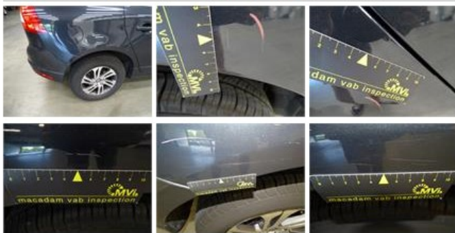
Wing F R, Bad repair, Acceptable
