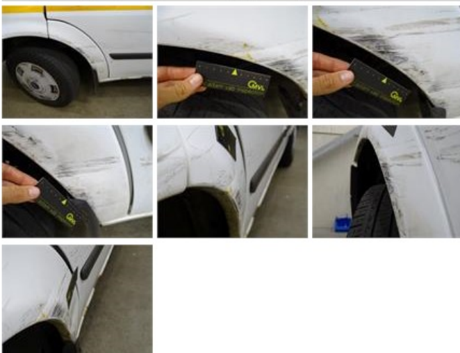
Sidewall RL (LCV), Dent(s) and scratch(es), It - Spot repair
