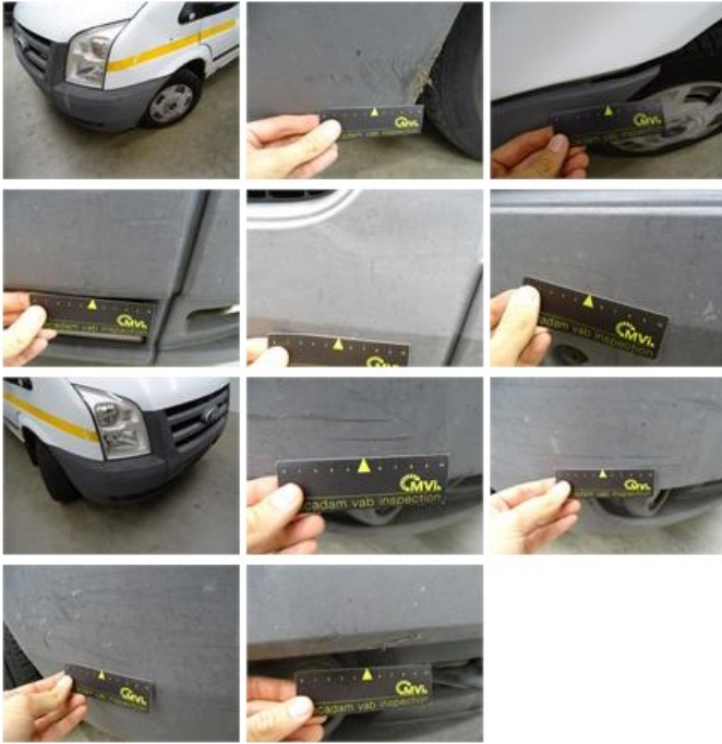
Door R R, Dent(s) and scratch(es), LI - Repair and paint (complete)
