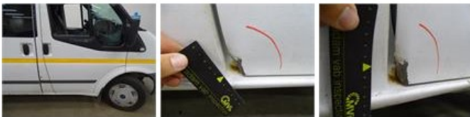
Central pillar R, Rust, LI - Repair and paint (complete)
