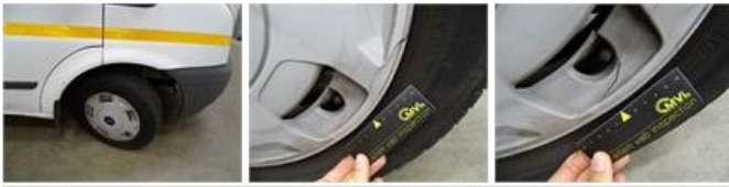
Bumper F, Scratch(es), Smart repair
