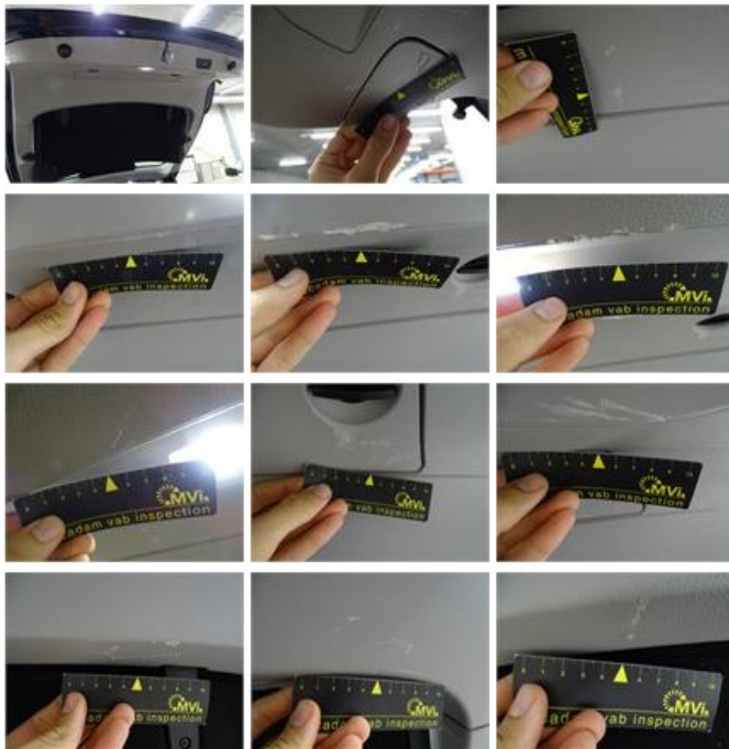
Door F R, Dent(s) and scratch(es), LI - Repair and paint (complete)
