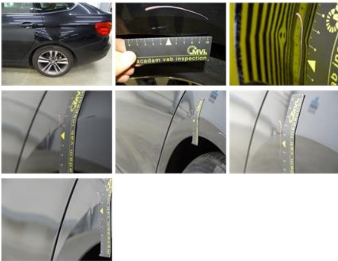
Bumper F, Scratch(es), LI - Repair and paint (complete) 211,80
