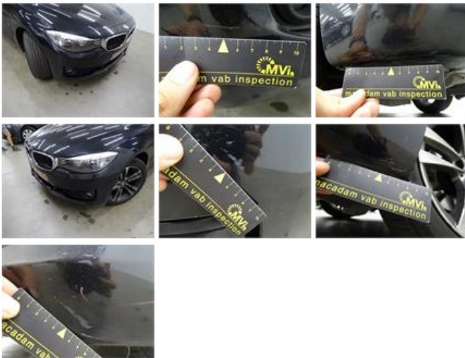
Door R R, Scratch(es), LI - Repair and paint (complete) 318,35
