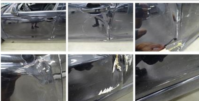
Door F L, Dent(s) and scratch(es), Le - Replace and paint 1270,21
