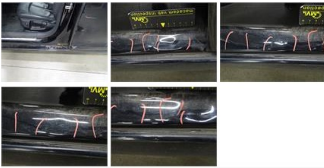
Door R R, Scratch(es), LI - Repair and paint (complete) 382,02
