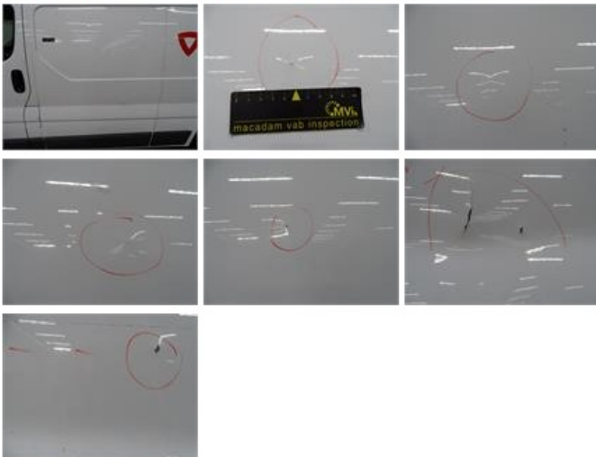
Trunk door R R, Dent(s) and scratch(es), It - Spot repair
