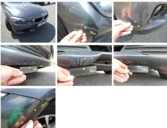
Bumper grille, Broken, E - Replace
