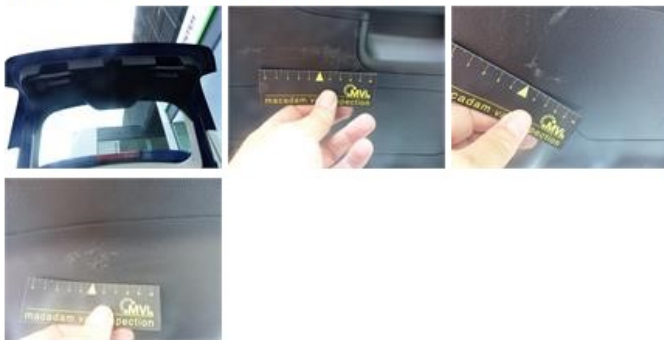
Wheel cover R R, Scratch(es), E - Replace
