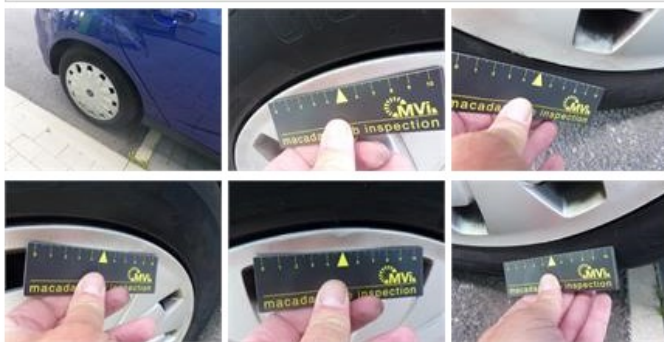
Wing R R, Dent(s) and scratch(es), Acceptable
