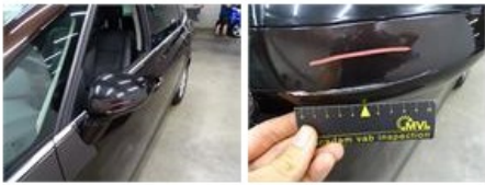
Sill outer L, Dent(s) and scratch(es), LI - Repair and paint (complete)
