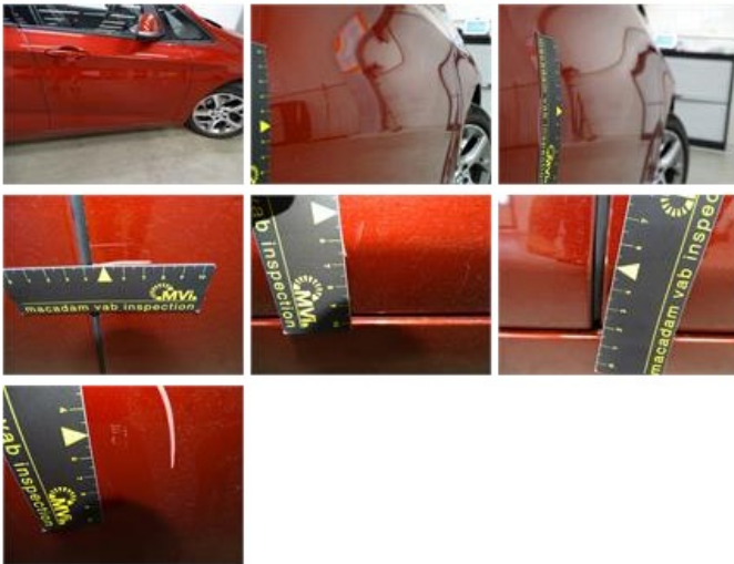
Alloy rim R R polished, Scratch(es), LI - Repair and paint (complete)
