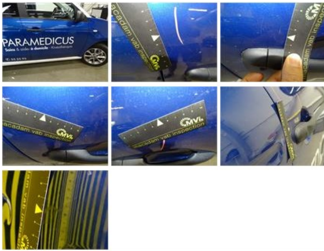
Rocker panel inner F L, Dent(s), LI - Repair and paint (complete)
