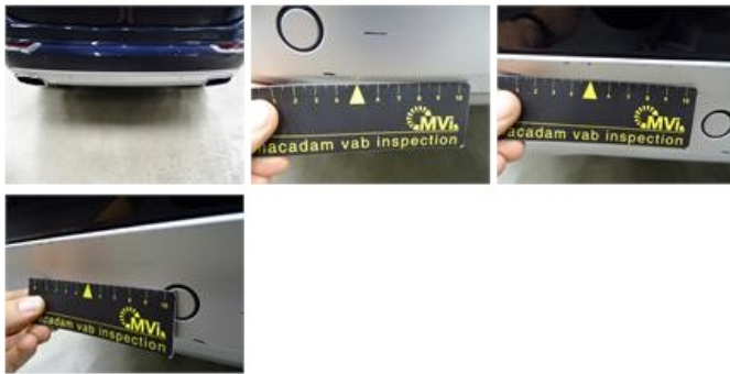
Bumper spoiler F, Dent(s) and scratch(es), It - Spot repair
