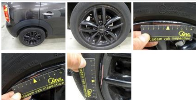
Bumper moulding R, Bad repair, E - Replace
