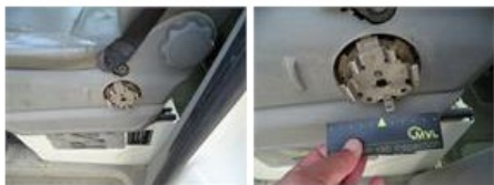
Seat cover F L, Damaged, E - Replace
