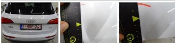
Tailgate, Dent(s) and scratch(es), LI - Repair and paint (complete)
