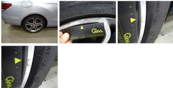
Tyre F L, Tear, E - Replace
