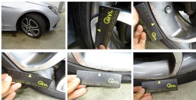
Alloy rim R L polished, Scratch(es), Acceptable
