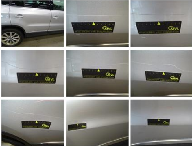
Roof pillar R, Scratch(es), Acceptable
