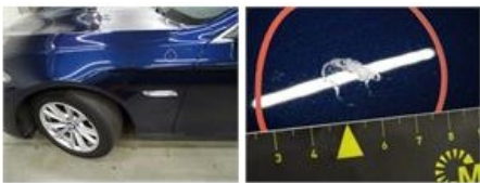
Door F L, Scratch(es), LI - Repair and paint (complete)
