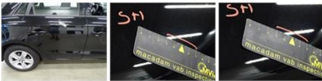
Door F R, Bad repair, Acceptable
