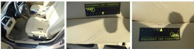
Seat cover F L, Worn, E - Replace
