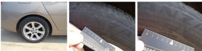
Tyre R L, Tear, E - Replace
