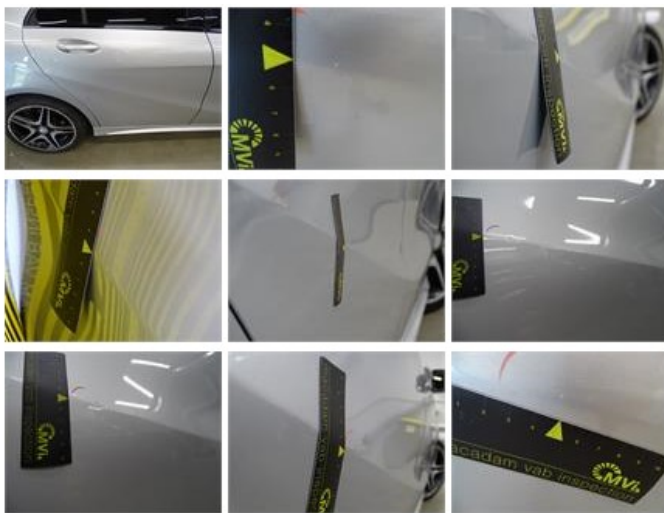
Bonnet, Dent(s) and scratch(es), LI - Repair and paint (complete)
