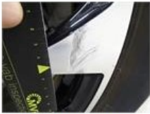
Sill outer R, Crack, Le - Replace and paint
