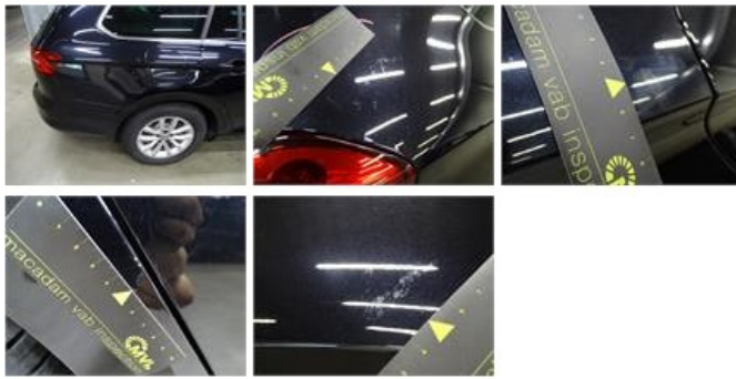
Door F R, Chemical polution, LI - Repair and paint (complete)
