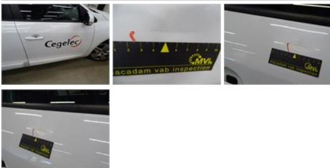
Sill outer L, Dent(s) and scratch(es), LI - Repair and paint (complete)
