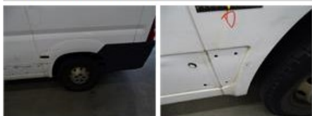
Sill outer R, Dent(s) and scratch(es), LI - Repair and paint (complete)
