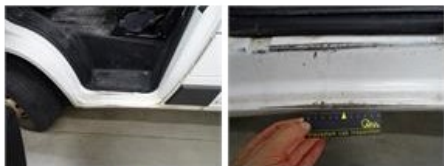
Wing trim R L, Missing, E - Replace
