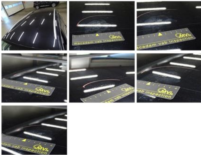
Sill outer L, Dent(s) and scratch(es), LI - Repair and paint (complete)
