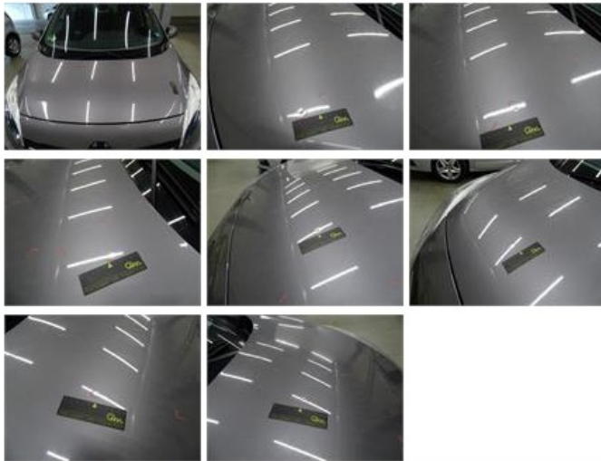
Roof, Hail damage, LI - Repair and paint (complete)
