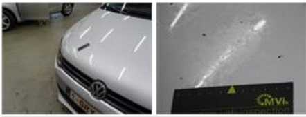
Roof, Dent(s), LI - Repair and paint (complete)
