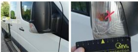
Door R R, Rust, LI - Repair and paint (complete)
