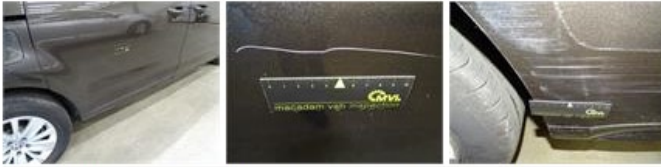
Door F R, Dent(s) and scratch(es), LI - Repair and paint (complete)
