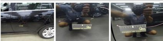
Door R R, Scratch(es), LI - Repair and paint (complete) 382,02
