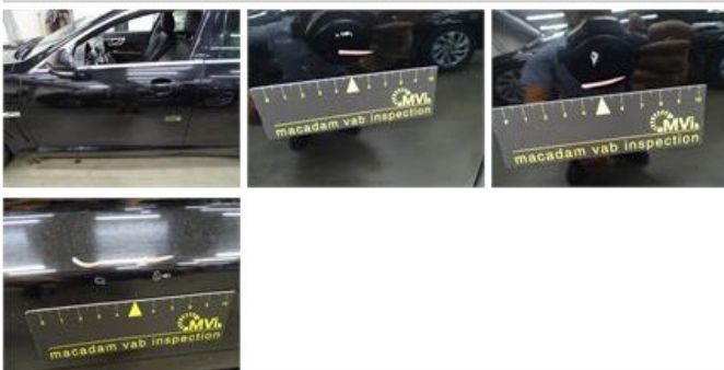
Door R L, Scratch(es), LI - Repair and paint (complete) 382,02
