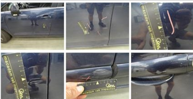
Wing F R, Deformed / Strained, LI - Repair and paint (complete)
