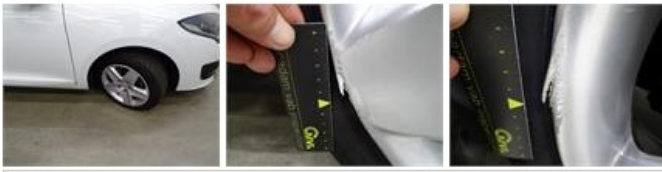
Bumper F, Crack, Le - Replace and paint
