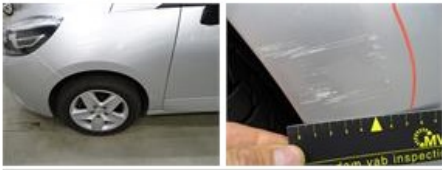
Wheel cover F R, Deformed / Strained, E - Replace
