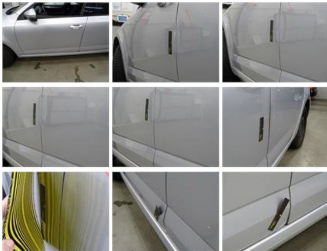
Door seal F L, Deformed / Strained, E - Replace
