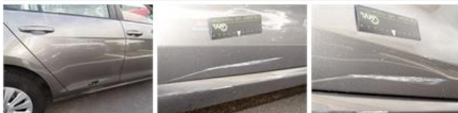
Wing R L, Dent(s) and scratch(es), LI - Repair and paint (partial)
