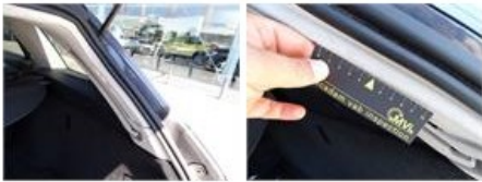
Rear roof pillar covering R, Hole, Smart repair
