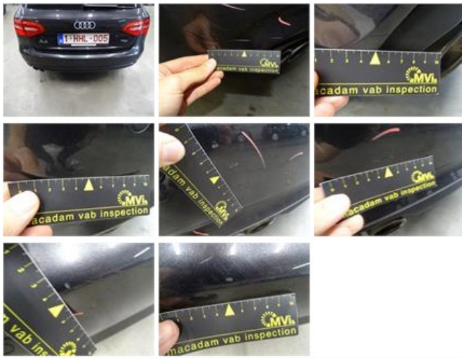
Protection plate M, Deformed / Strained, E - Replace
