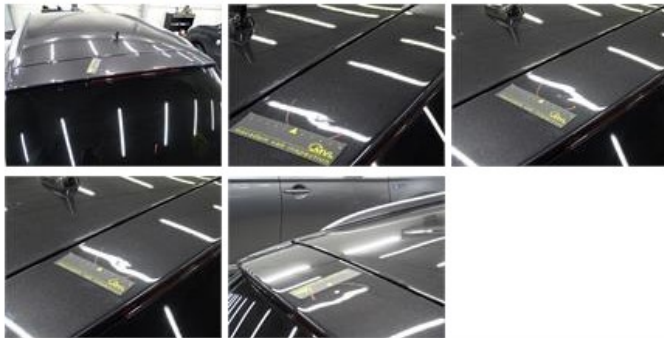
Rear window, Scratch(es), Acceptable
