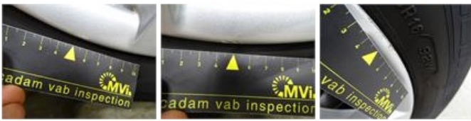
Bonnet, Dent(s), PDR - Paintless dent repair
