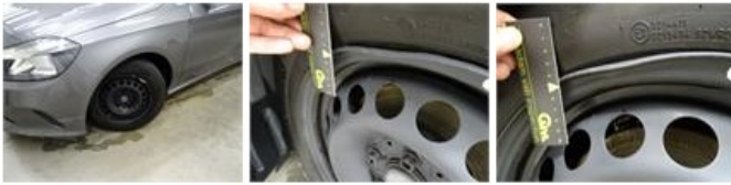
Wheel cover R L, Scratch(es), E - Replace
