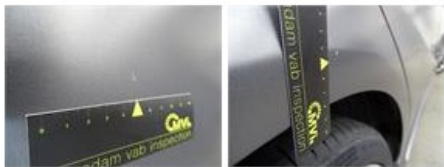
Bumper R, Dent(s) and scratch(es), LI - Repair and paint (complete)
