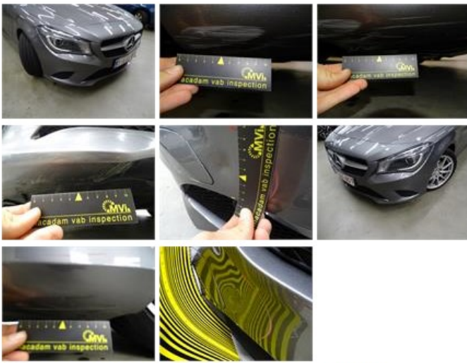
Door R L, Dent(s) and scratch(es), LI - Repair and paint (complete)
