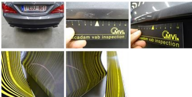
Rear window, Scratch(es), Acceptable
