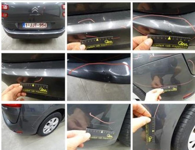
Tailgate, Scratch(es), LI - Repair and paint (complete)
