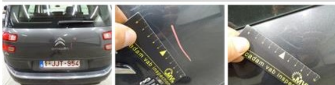
Tailgate, Scratch(es), LI - Repair and paint (complete)
