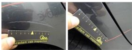
Door R R, Scratch(es), LI - Repair and paint (complete)
