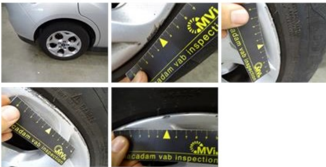
Door F L, Dent(s), LI - Repair and paint (complete)
