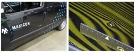
Sidewall RL (LCV), Dent(s) and scratch(es), It - Spot repair
